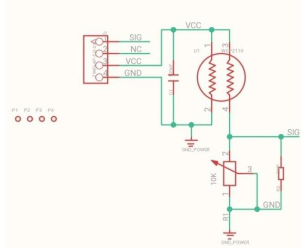
Figure III. WSP 2110 SENSOR CIRCUIT DIAGRAM
